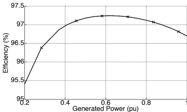
Figure 5: Efficiency versus load for 6 MW Brushless DFIG (Frame: 1200)
