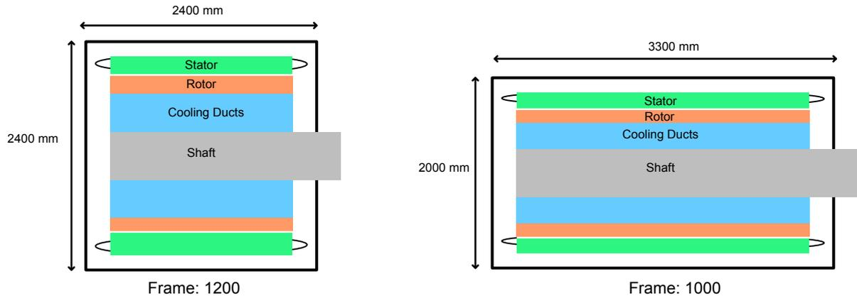
Figure 3: Physical dimensions of 6 MW Brushless DFIG with different frame sizes
