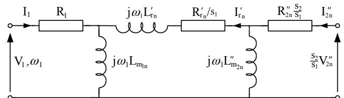
Figure 4: Per-phase equivalent circuit for the Brushless DFIG
