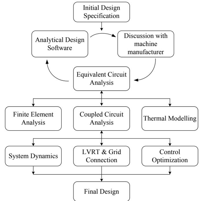
Figure 2: Design procedure for the Brushless DFIG system
