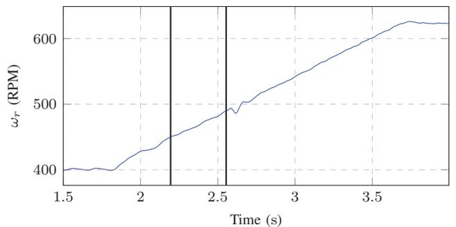
**Figure 2.** Rotor speed profile for experimental grid synchronization. First vertical line indicates start of grid synchronization routine. The second indicates the point of synchronization.
