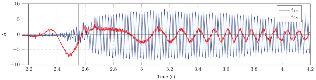
**Figure 4.**  $a$ -phase currents for the PW and CW
