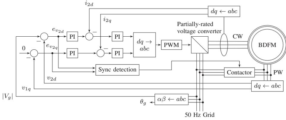
Figure 1. Grid synchronization setup
