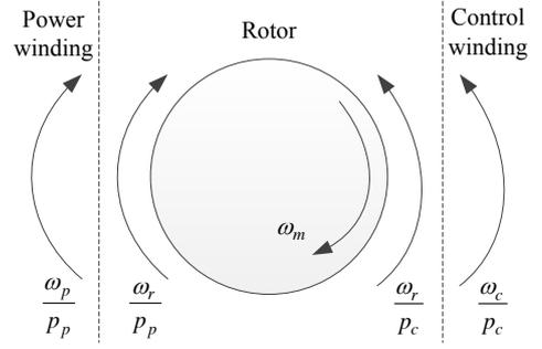
Fig. 3. Rotating speed of stator and rotor fundamental fields in BDFIM
