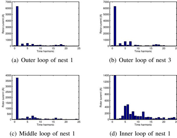
Fig. 5. Time FFT of rotor currents
