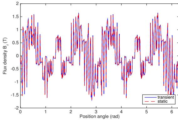
Fig. 6. Total air-gap flux density in the radial direction
