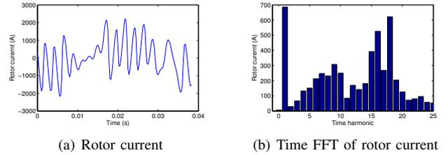
Fig. 7. Rotor current and its time FFT - loop span  $3^\circ$
