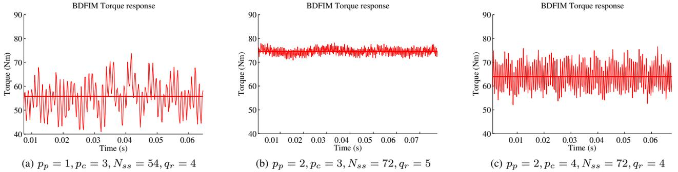
Fig. 8. Torque response, including main torque
