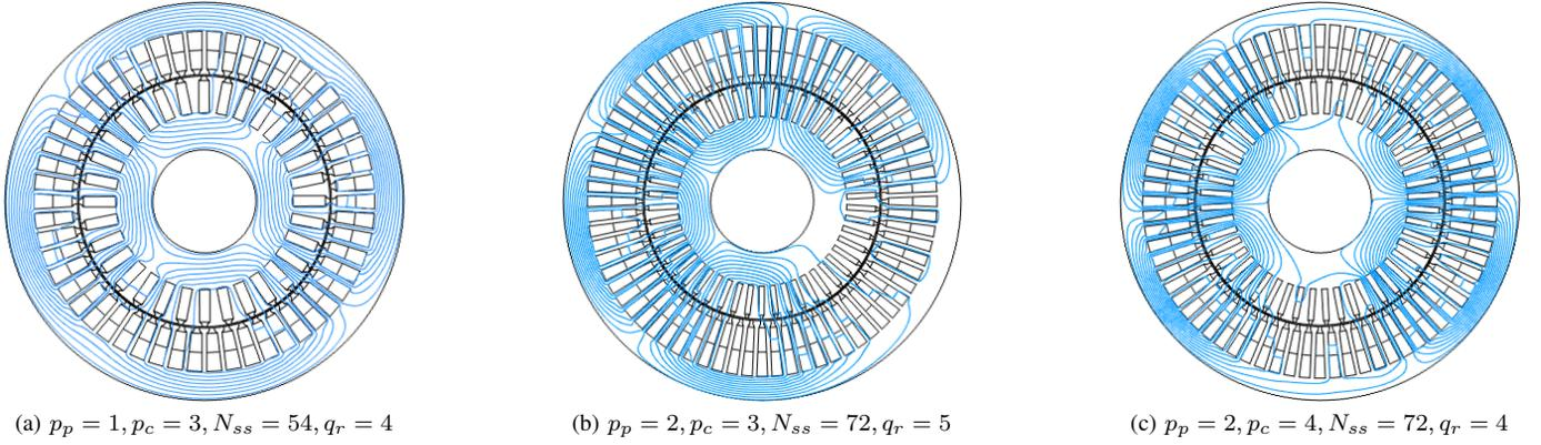
Fig. 4. Optimized machine design geometries for different construction variations (including magnetic field lines)
