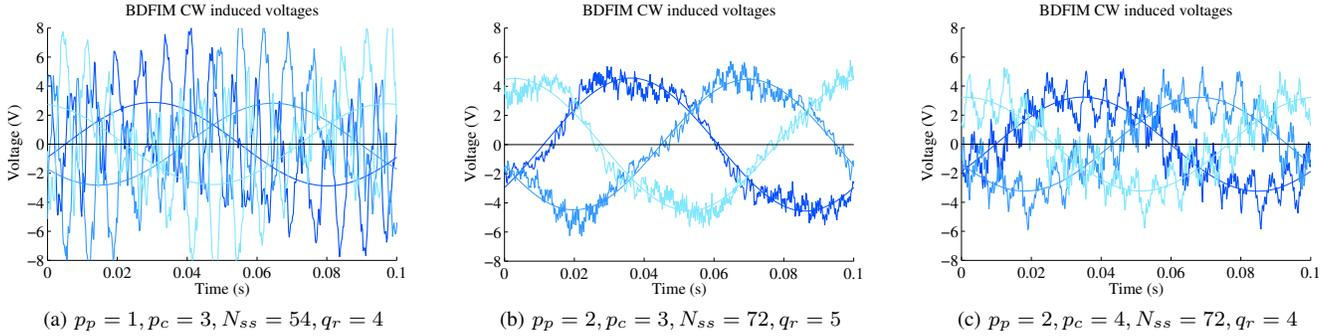
Fig. 6. Single-turn induced phase voltages in the CW, including main harmonic components
