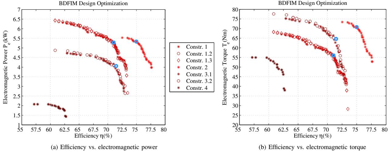
Fig. 3. BDFIM design optimization results for different construction variations
