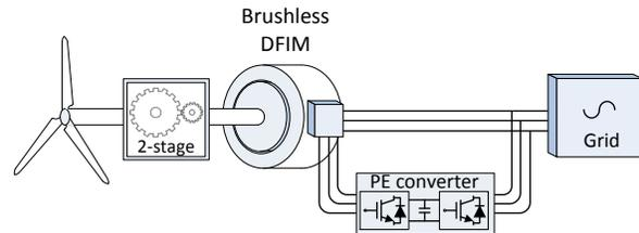
Fig. 1. Brushless DFIM incorporated in a wind turbine drive-train.
