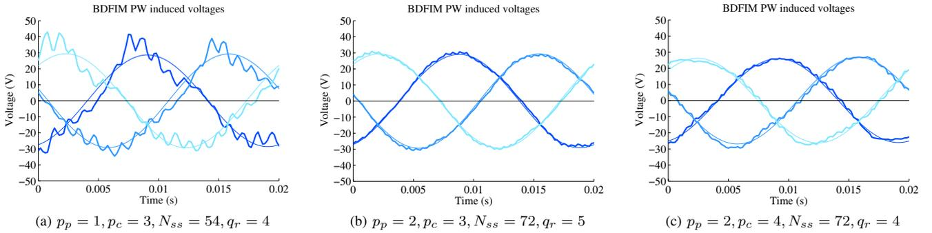
Fig. 5. Single-turn induced phase voltages in the PW, including main harmonic components
