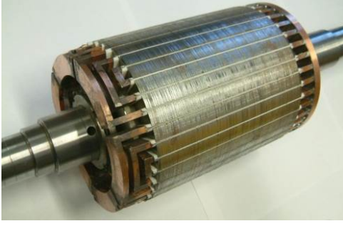
Fig. 1. Nested-loop structure of the BDFIM considered [2]
