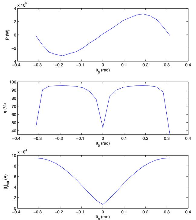
Fig. 7. Power, efficiency and total rotor current as function of  $\theta_0$ .
