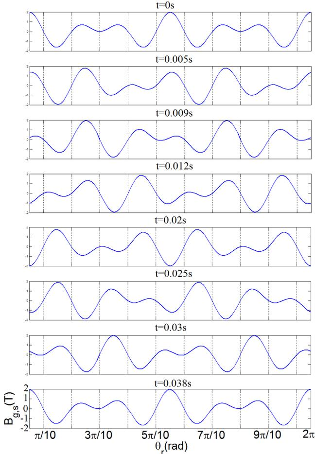
Fig. 2. Flux density distribution for a BDFIM with 6 and 4 pole pairs.
