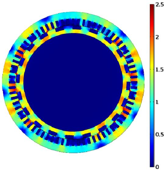
Fig. 4. 2D Patterns of flux densities of the analyzed BDFIM.
