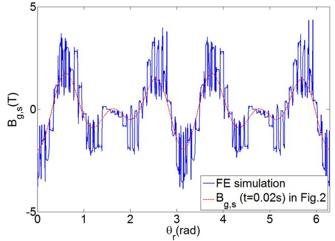
Fig. 6. Comparison of an analytical and a finite element calculation of the radial components of the air gap flux density due to the stator currents.
