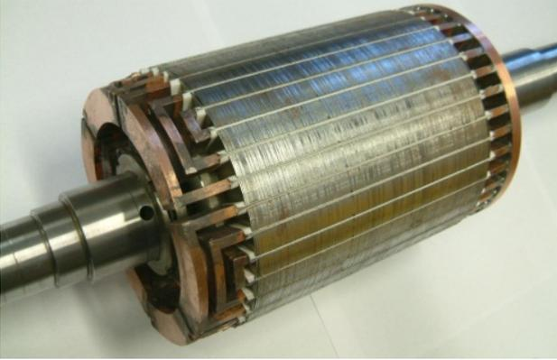
Fig. 1. The rotor of a brushless DFIG with 6 nested loops, as used in a machine with a stator with a 4-pole and an 8-pole winding, reproduced from [3].
