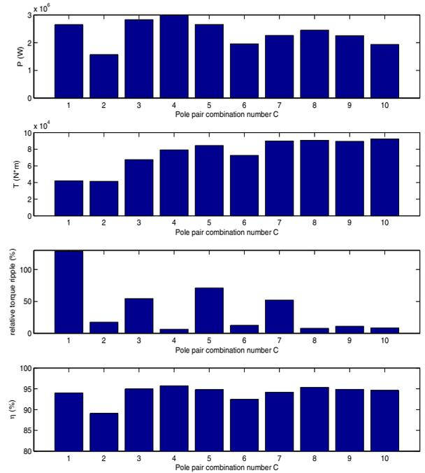
Fig. 8. Power, torque, torque ripple, efficiency for the various pole pair combinations.
