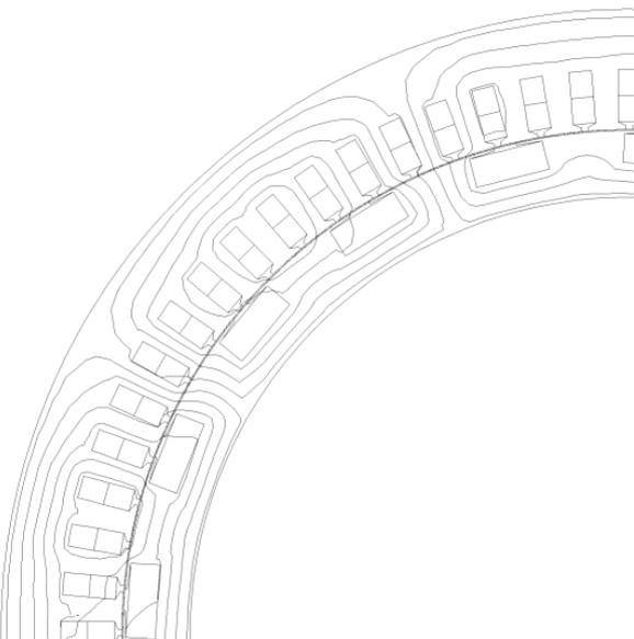
Fig. 5. 2D Flux lines of the analyzed BDFIM.
