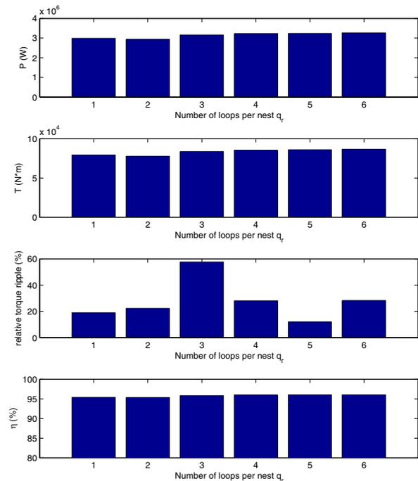
Fig. 9. Power, torque, torque ripple and efficiency for various loops per nest.
